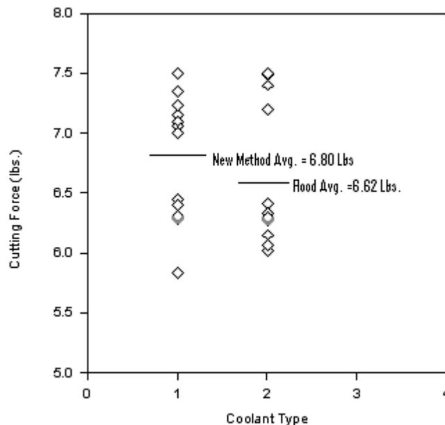
**Figure 2** Scatter Plot Comparing Cutting Forces From the New System and Flood Cooling
