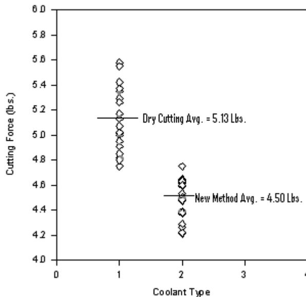
**Figure 1** Scatter Plot Comparing Cutting Forces From Dry Cutting and the New Method
