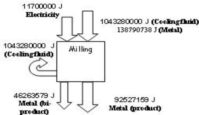
Figure 7: Exergy accounting of the milling process
