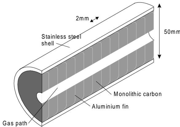
Figure 2. Generator geometry.
