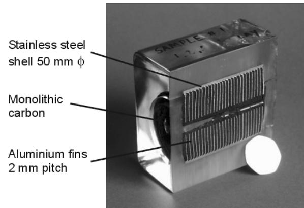
Figure 3. Generator section (total generator length is 1m).
