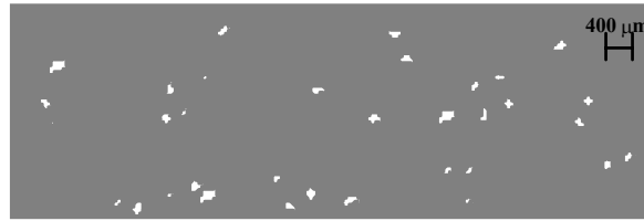
Figure 17. Distribution of PUR-HMA particles (white) in PP (grey) in PP/PUR-HMA 92/8.
