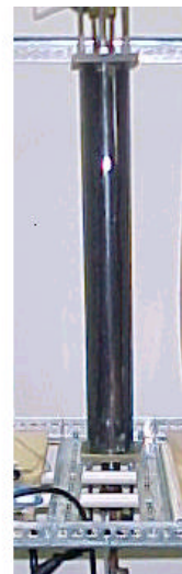
Figure 2. A schematic drawing of the single tube condensation apparatus (left) Figure 3. A photograph of the single tube condenser (right)
